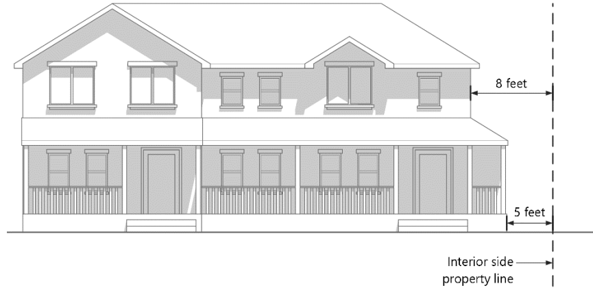
Figure 4-3. Two-Story Attached Units on Continuous Lots
